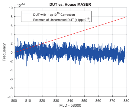
Fig. 11. MASER DUT Frequency Measurements with -1\text{pp}10^{15}/\text{Day} Correction
